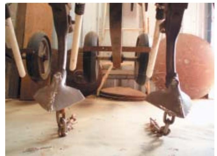
*A 28 run combine fitted with wide but steep points for furrow sowing*
